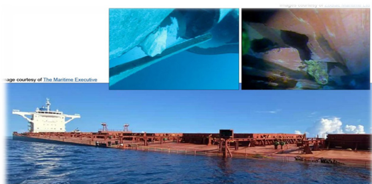
Figure 1: Indian Partnership partially submerged at anchor off Misool Island and (insets) rock fragments embedded in the hull
