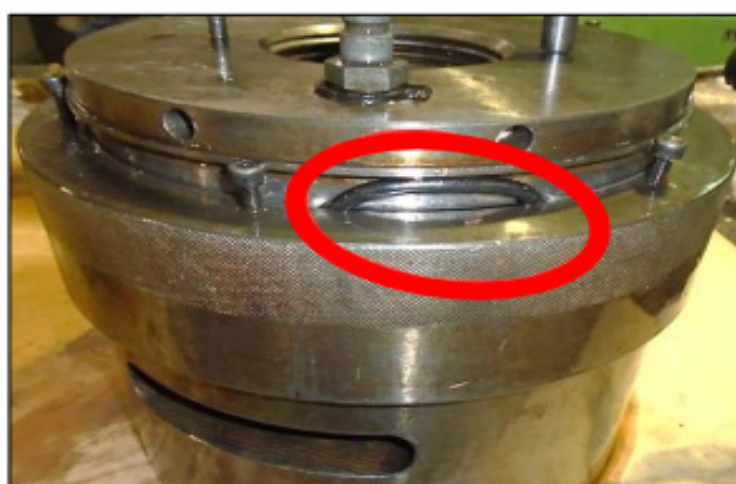
Figure 6: Displaced upper sealing ring
