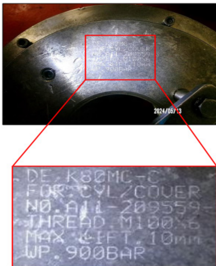
Figure 5: Maximum working pressure and lift, stamped on the hydraulic jack assembly
